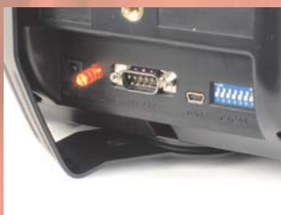
Red LED Power lamp, USB port for zone programming & volume adjustment.
