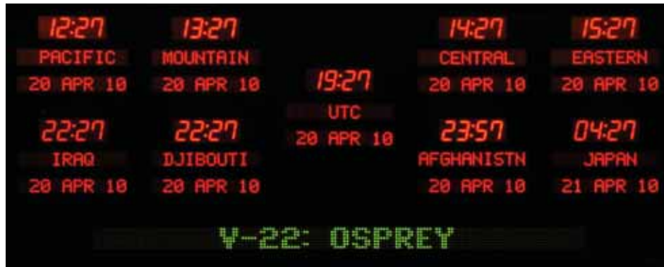
Model 7329A - 1.8" time, 1.2" zone labels & character date, 9 zone with a 48" tri color moving message display
